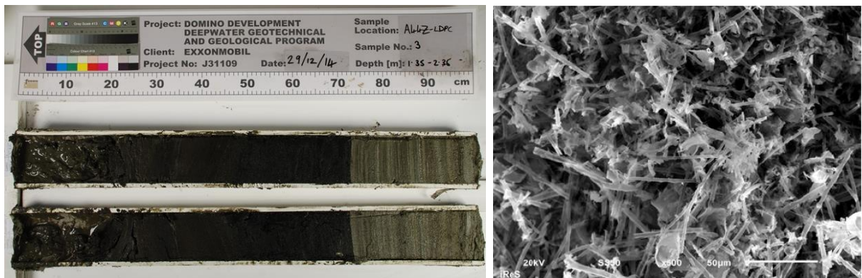
Figure 3.2: (Left) Sample photograph from A44Z-LDPC (Fugro, 2015c) showing GU2 black organic clay (sapropel) between 1.35 m and 2.05 m BML and (Right) a scanning electron microscope image of abundant fibrous tubular biogenic structures from GU2 organic clay (sapropel)
